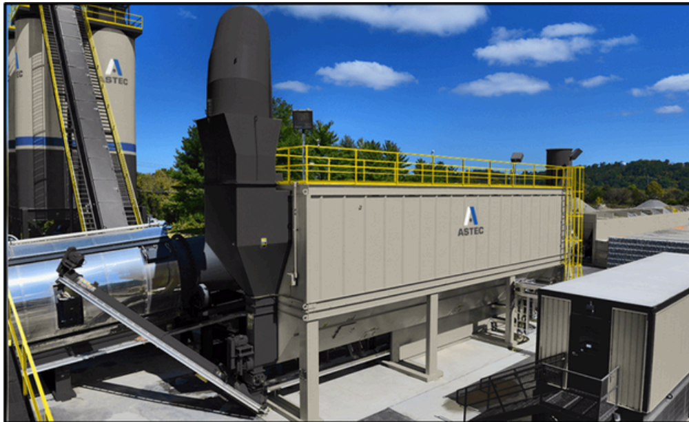
ASTEC Pulse Jet Baghouse (Photo courtesy of ASTEC)
