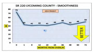
Figure 2 Site 3 SR 220 Before and after ride numbers on full depth asphalt pavement.
