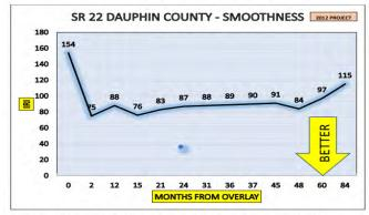
Figure 3 Site 1 SR 22 Before and after ride numbers on jointed concrete pavement.
