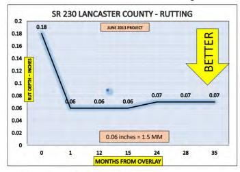
Figure 1 Site 2 SR 230 Before and after rut depths.
