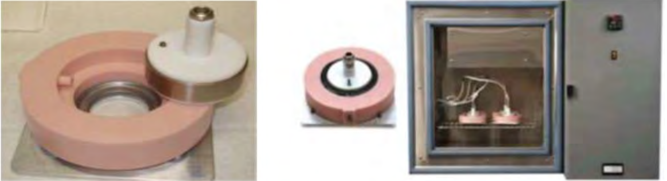
Figure 2: ABCD setup: Temperature Chamber; Filled & Empty Ring (King, 2007).
