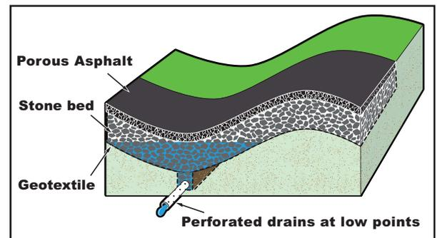
plants can easily prepare the mix and general paving contractors can install it. While modified asphalts are often used, these are not always necessary or practical.
