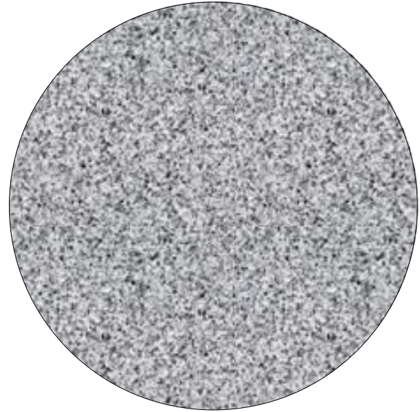
More proportional representation of ~10 \mu m binder film on a #4 aggregate
